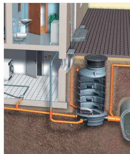
■ Example for underground installation
